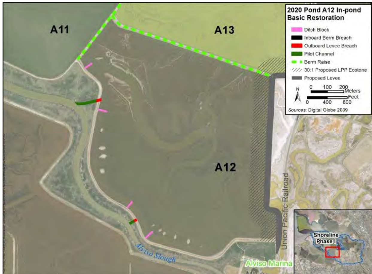
Diagram 2. In-Pond Preparation for Breaching of Pond A12.
