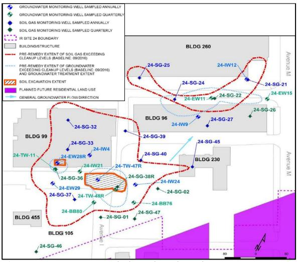
Figure 2. Site 24 excavation areas and soil gas and groundwater plumes
