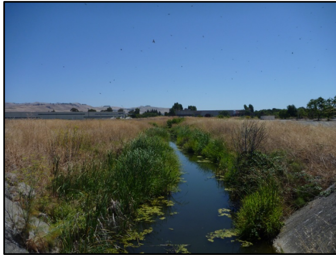
Photo 5-3: Fagan Creek maintenance reach, looking upstream from the inlet of the runway culvert, showing channel roughness.
