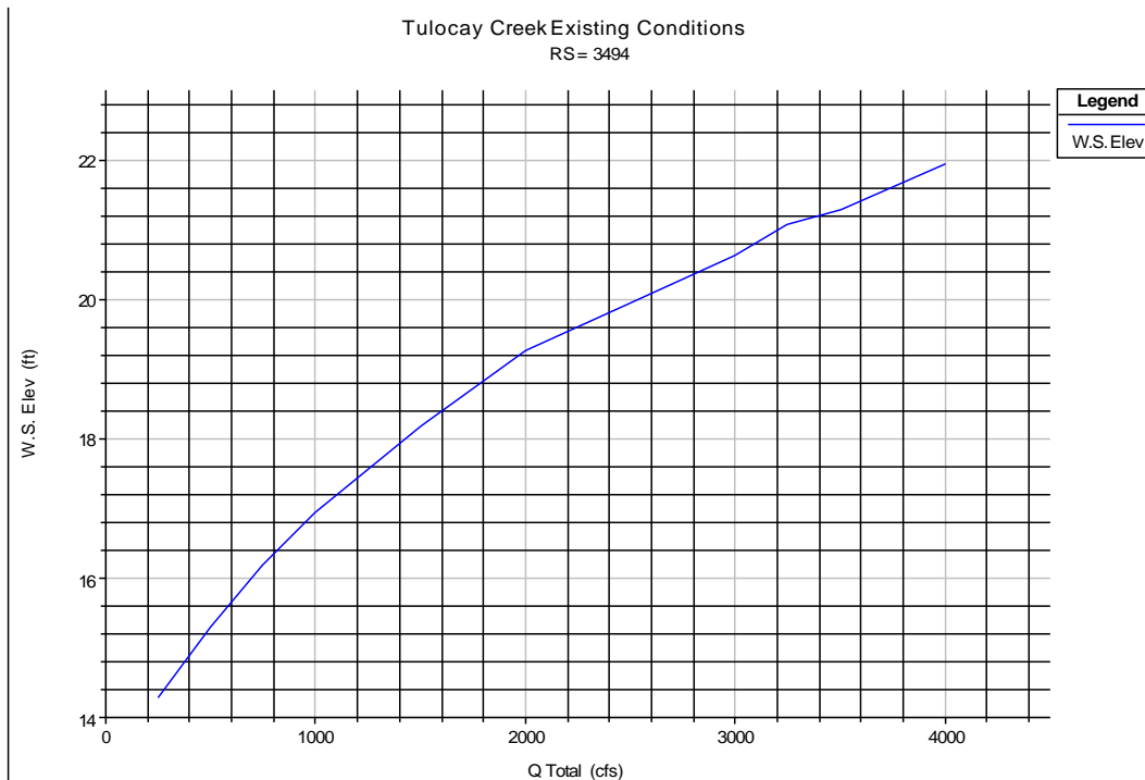
Figure 1. Stage-discharge rating for Tulucay Creek Reach 1, obtained from HEC-RAS analysis.
