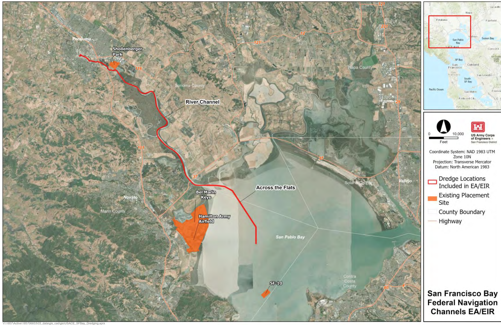
Figure 1-10. Dredge Locations and Material Placement Areas for Petaluma River Channel
