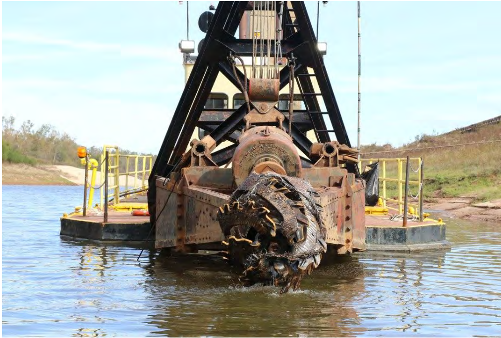
Figure 2-3. Example of a Cutterhead-Type Dredge
