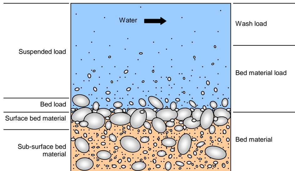
**Figure 13. Sediment transport and Bed Material Definitions**
