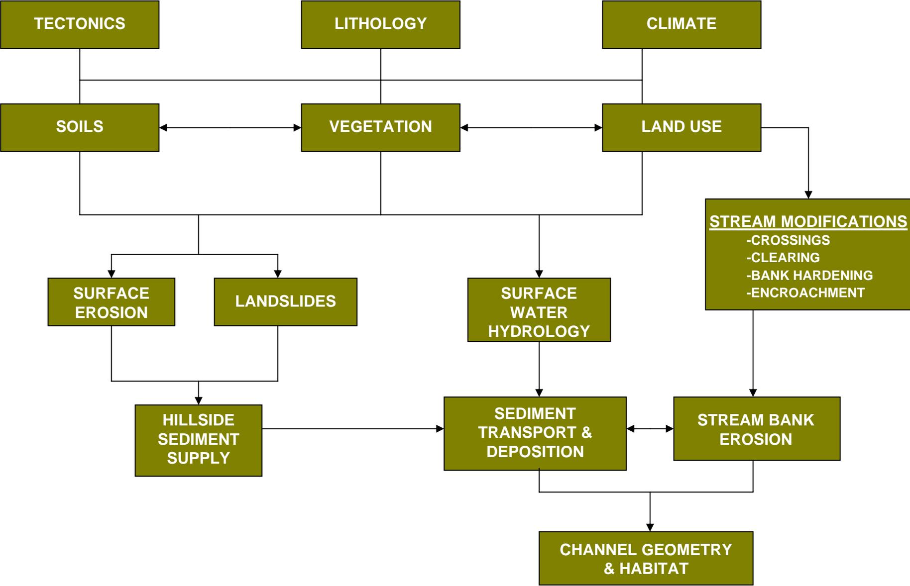
FIGURE 10. Conceptual Model of Erosion in San Francisquito Creek
