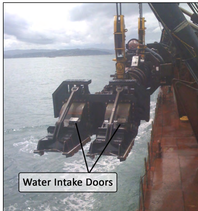
Figure 2-3 Essayons Drag Head and Water Intake Doors
