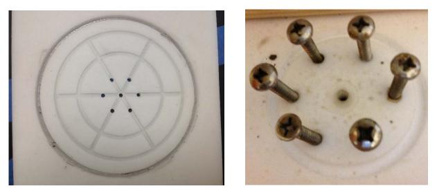
Figure 3. Teflon Column Cap with Drainage Veins and Holes (left) and Stainless Steel Throttling Screws (right)
