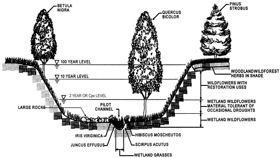
**Figure A.4 Section of Typical Shallow Extended Detention Wetland System**
