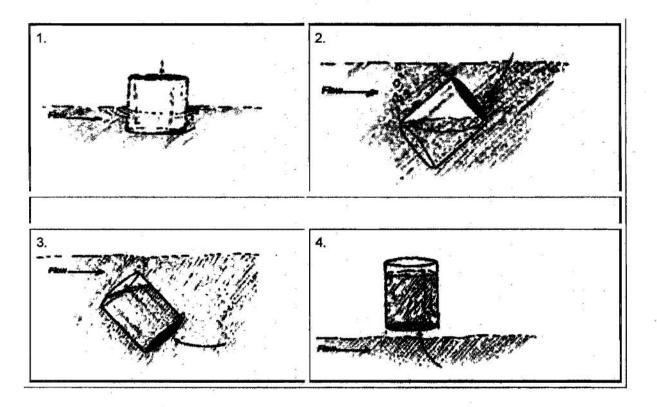
Taking a water sample. Turn the bottle into the current and scoop in an upstream direction.
