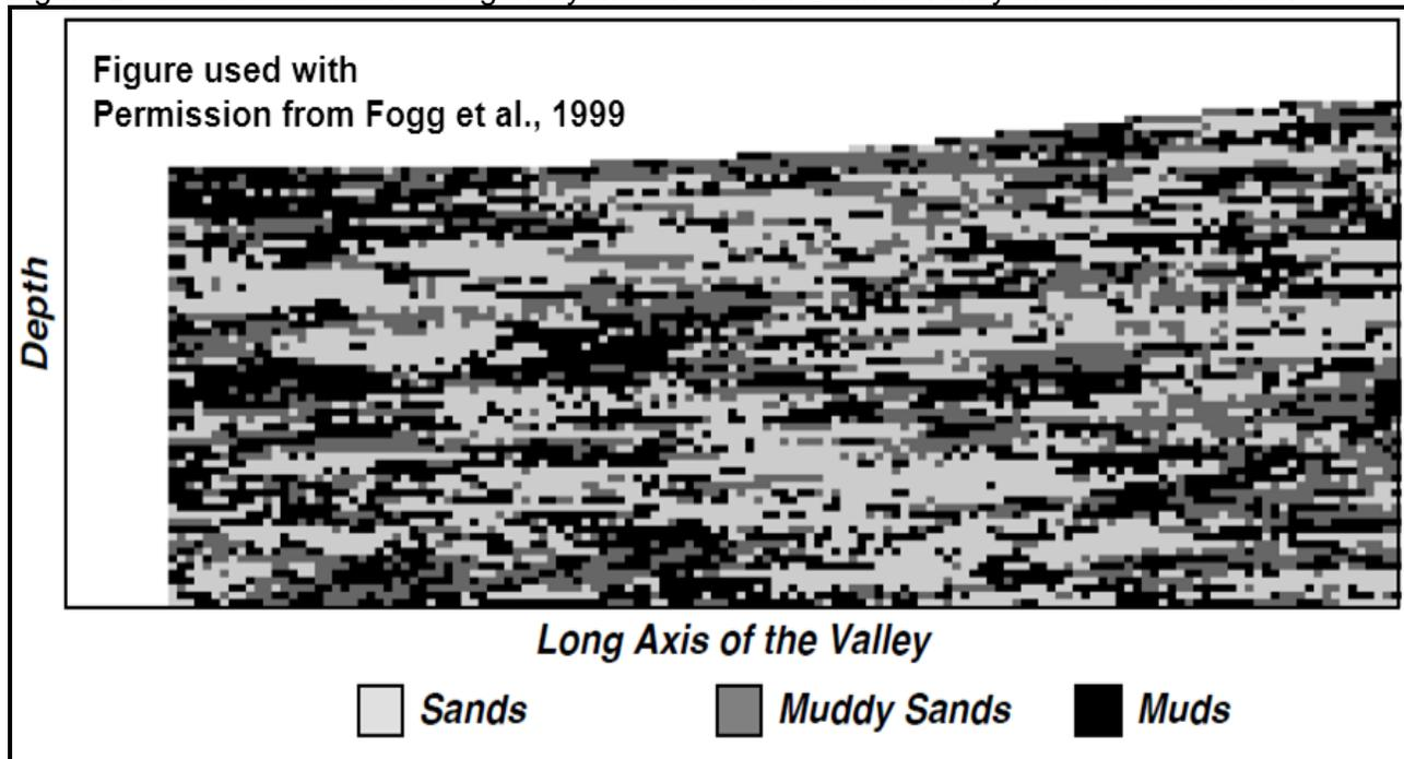
Figure 2-20 illustrates that shallow, laterally-discontinuous high permeability facies (channel belt sands and gravels) locally occur at very shallow depths (5 to 20 feet below ground surface) in the basin floor reaches of the lowermost Salinas Valley. These shallow, discontinuous permeable strata would be expected to be potential zones for perched groundwater horizons, and conduits for shallow groundwater flow and baseflow contributions to streams.
