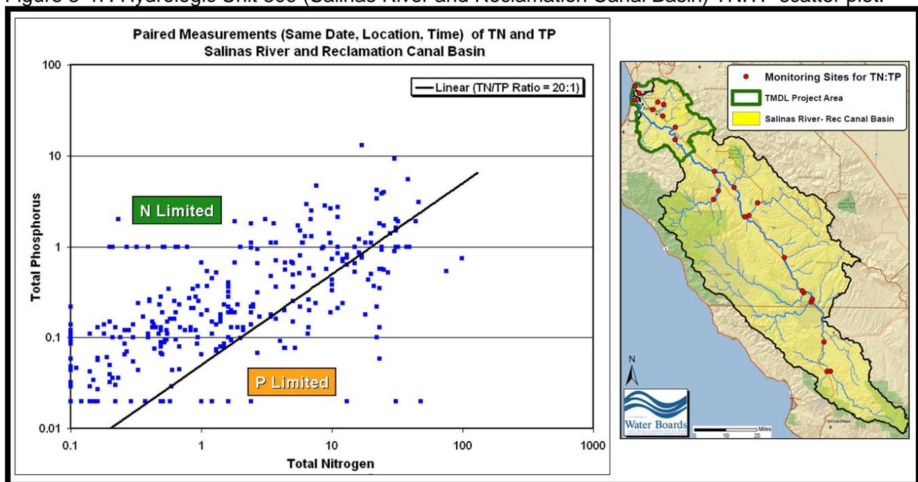
Figure 3-48. Water column TN:TP ratios (geomean of individual monitoring site samples).
