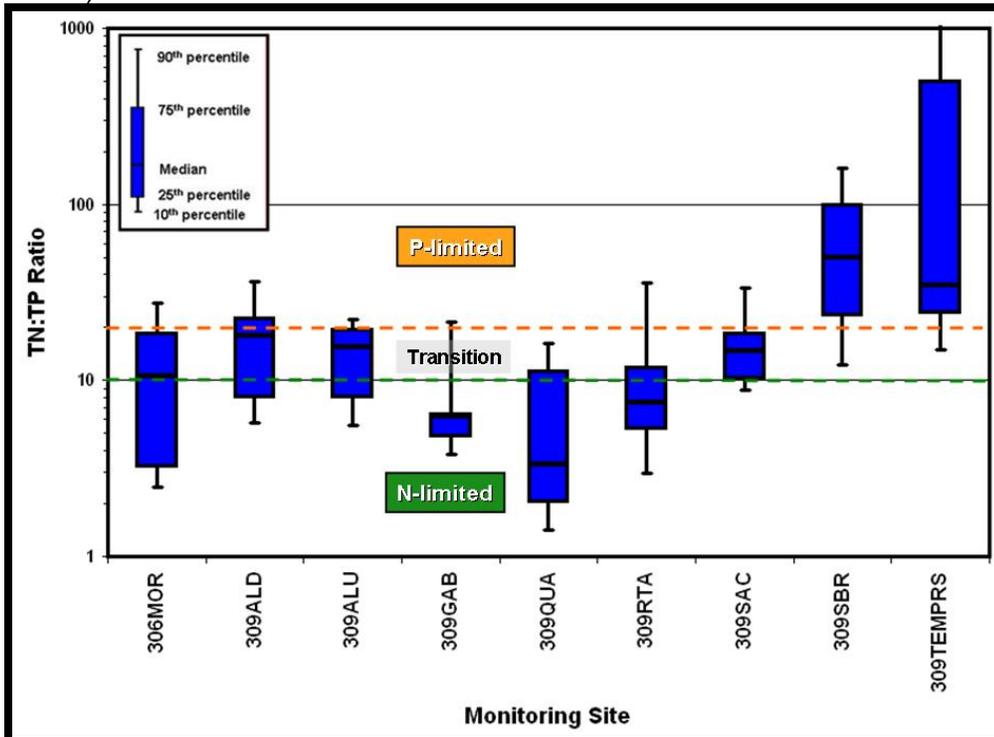
Table 3-22. Nutrient limitation determination for sites in TMDL project area.
