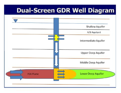
The process creates a local groundwater barrier in the lower deep aquifer to reduce the potential for perchlorate to flow towards the north were the City of Morgan Hill's (City) municipal wells pump from the lower deep aquifer. The GDR technology is a green technology that promises to locally cleanup and control perchlorate without the need for electric or hydrocarbon energy to operate pumps or for the construction of treatment system pipelines.
