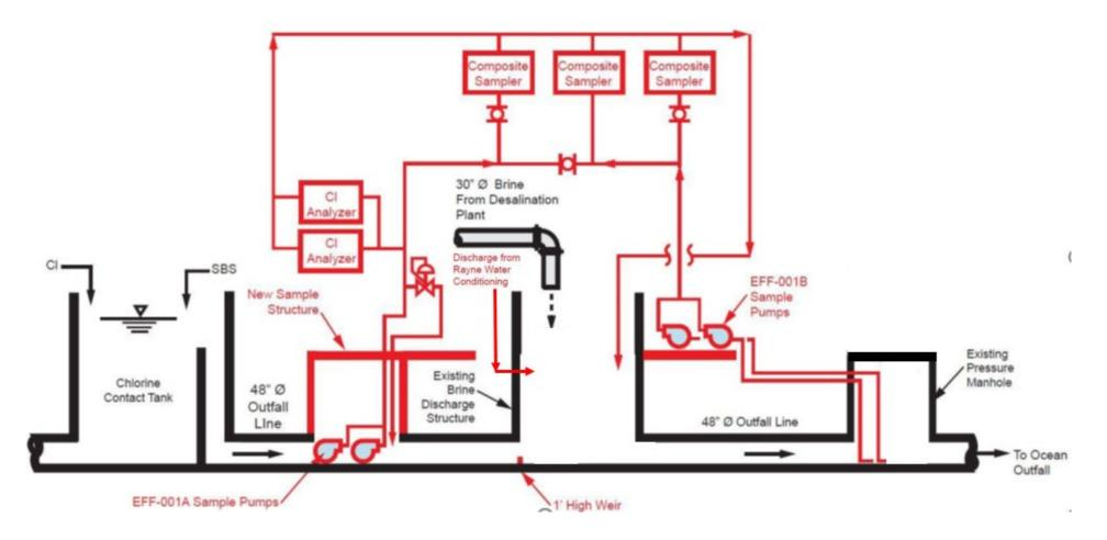
Figure C-2. Reconstructed Effluent Sampling Location
