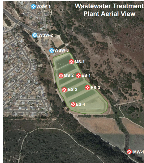
Figure B – Example aerial photograph of a Wastewater System. Location of water supply wells labeled with blue crosses. Location of monitoring well labeled with a red cross. Additional maps would be needed to show other system components.
