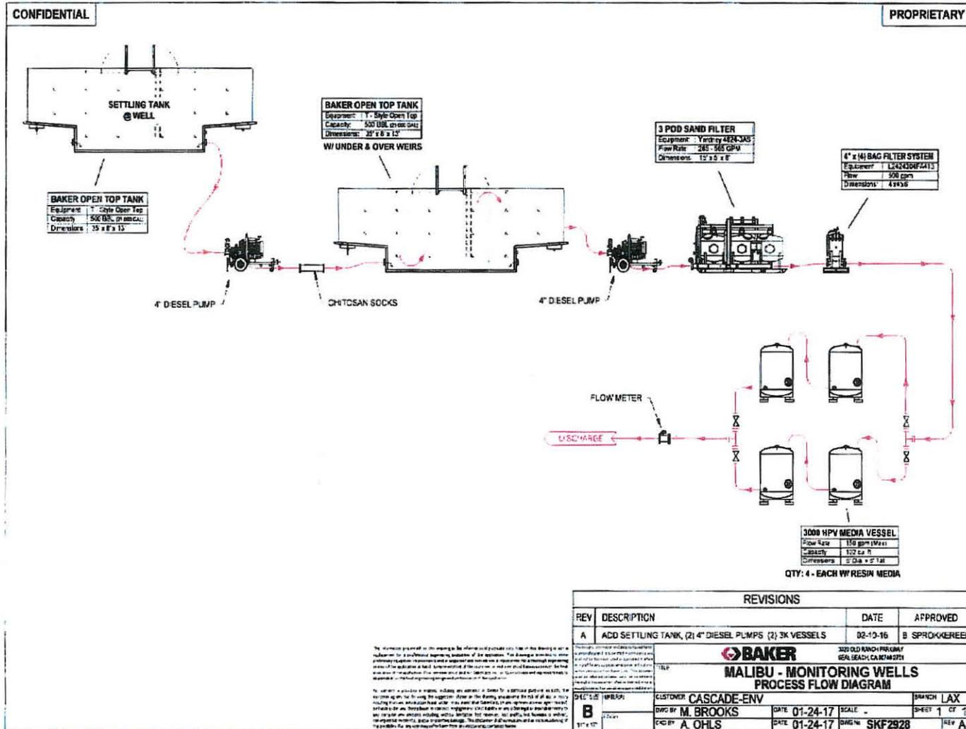
Figure 2. Treatment Schematic
