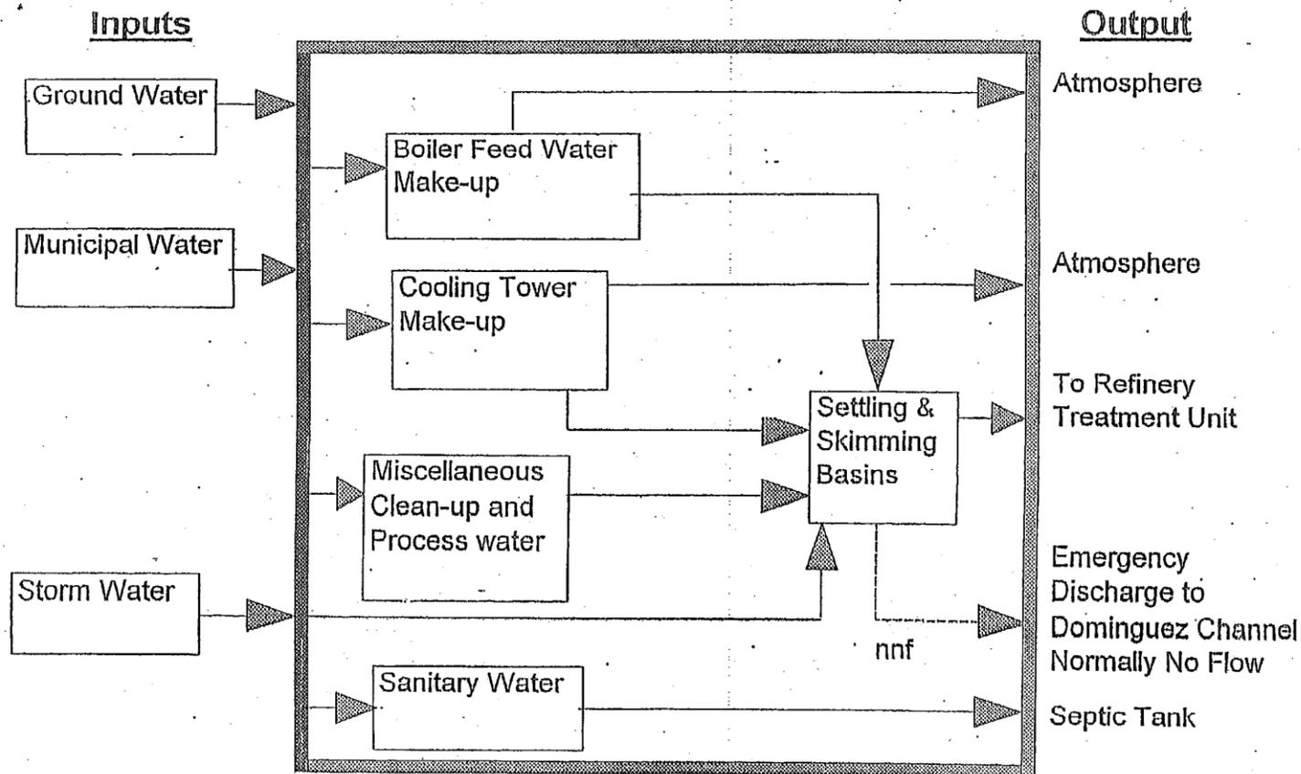
SRP WASTEWATER FLOW TO SETTLING & EFFLUENT BASINS
