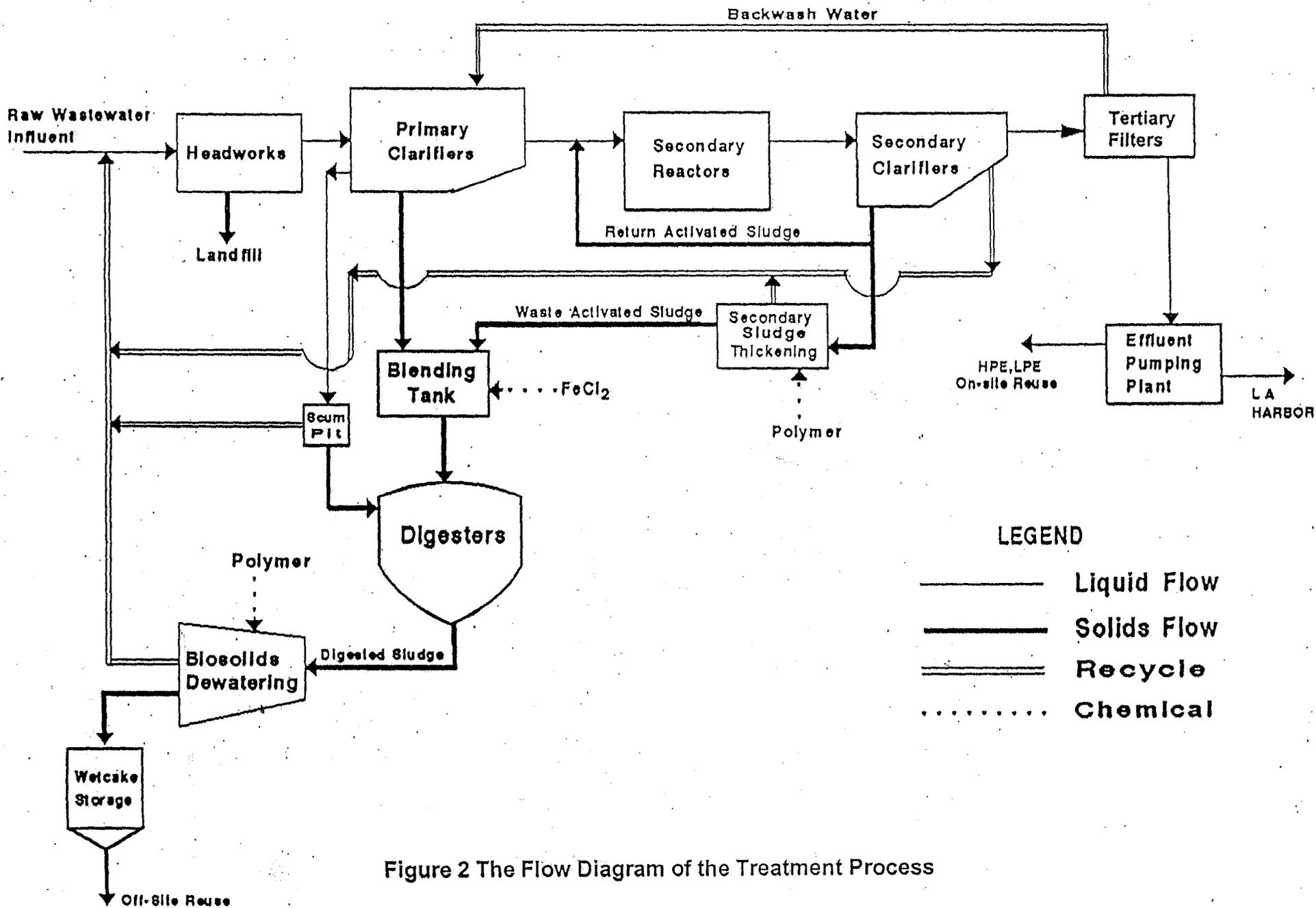
Figure 2 The Flow Diagram of the Treatment Process
