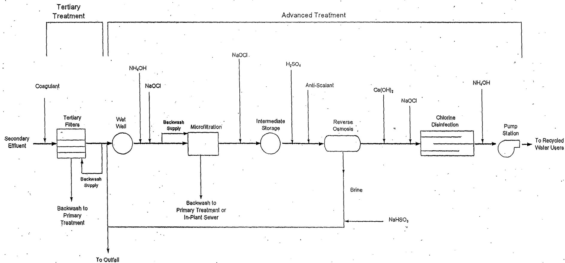
Figure 3 The Schematic of the Treatment Process for Phase I-AWTF
