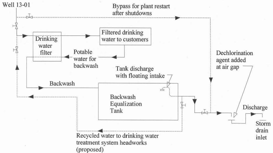
**Figure 2. Treatment Schematic**
