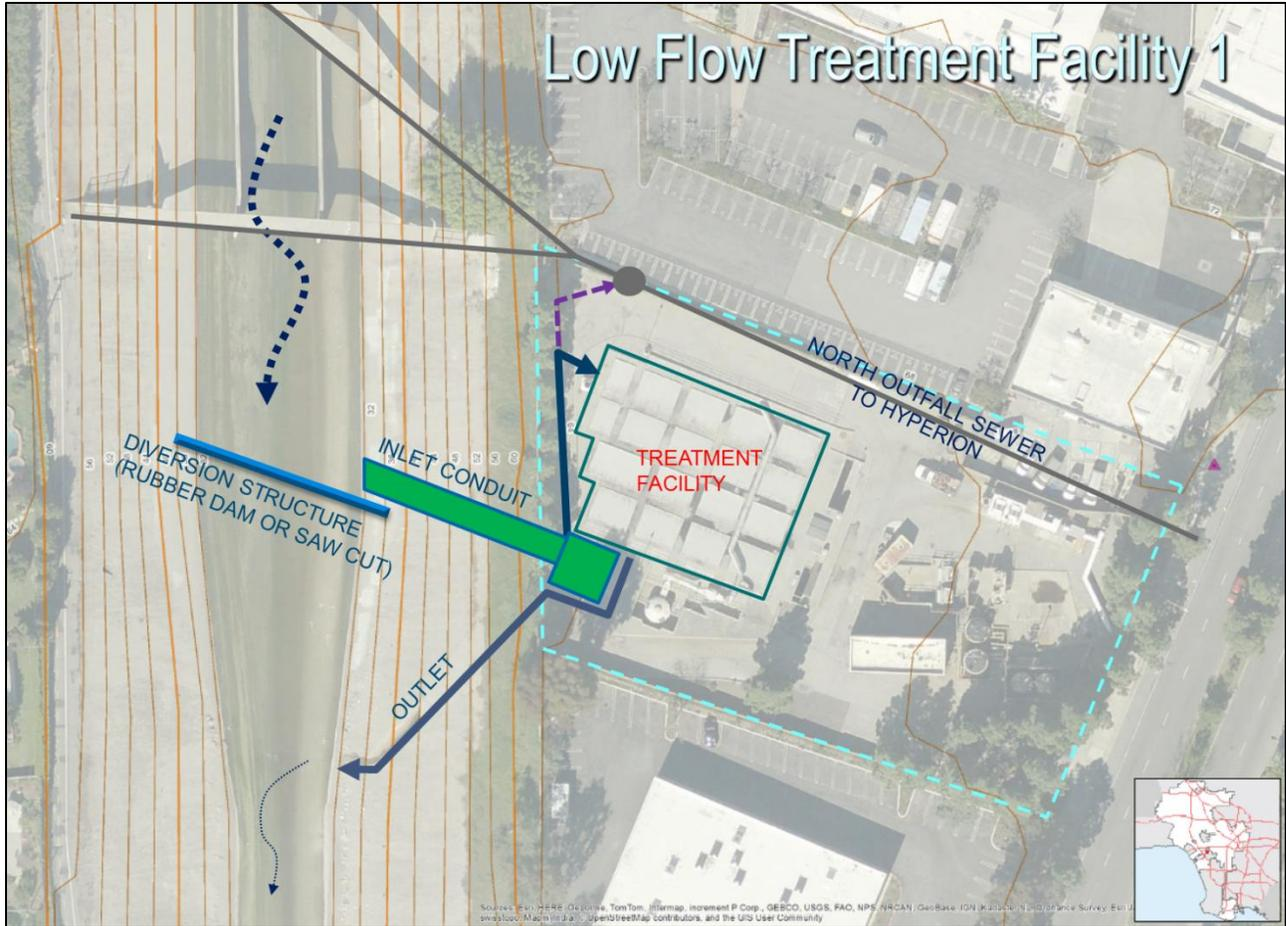
Figure 7. Plan View of the LFTF #1
