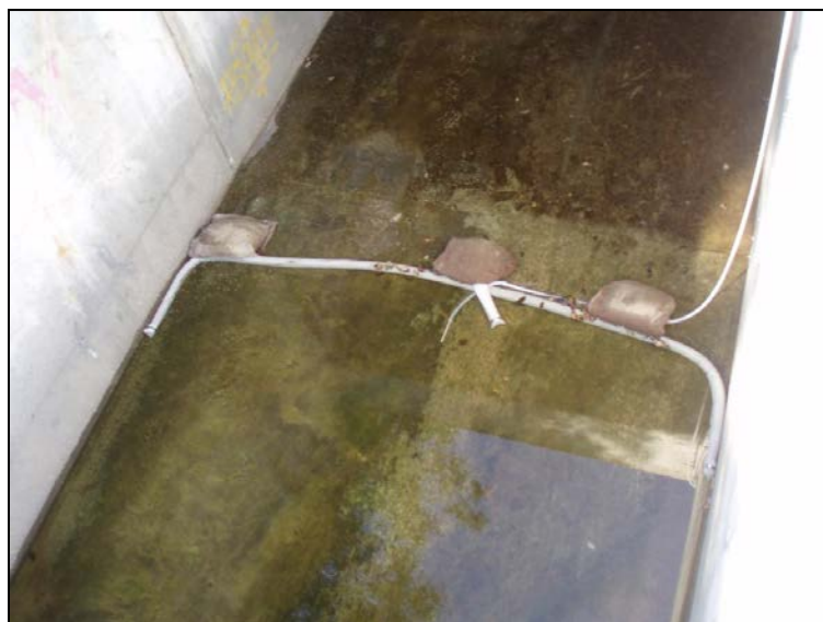
Figure 9-8. Typical Wet-Season, Dry-Weather Sampling Configuration
