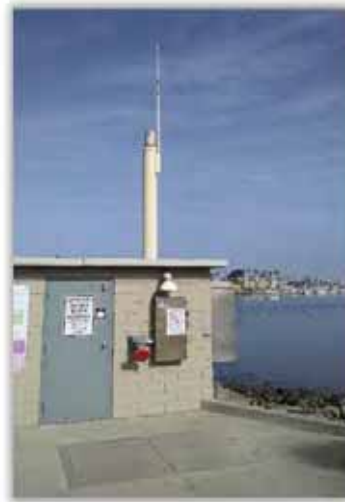
Stand pipe rain gage on roof of pump house (Provided by the County)
