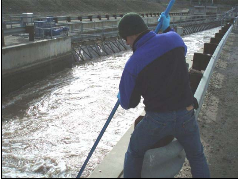
Figure 9-7. Grab Sampling Using Extended-Reach Swing Sampler
