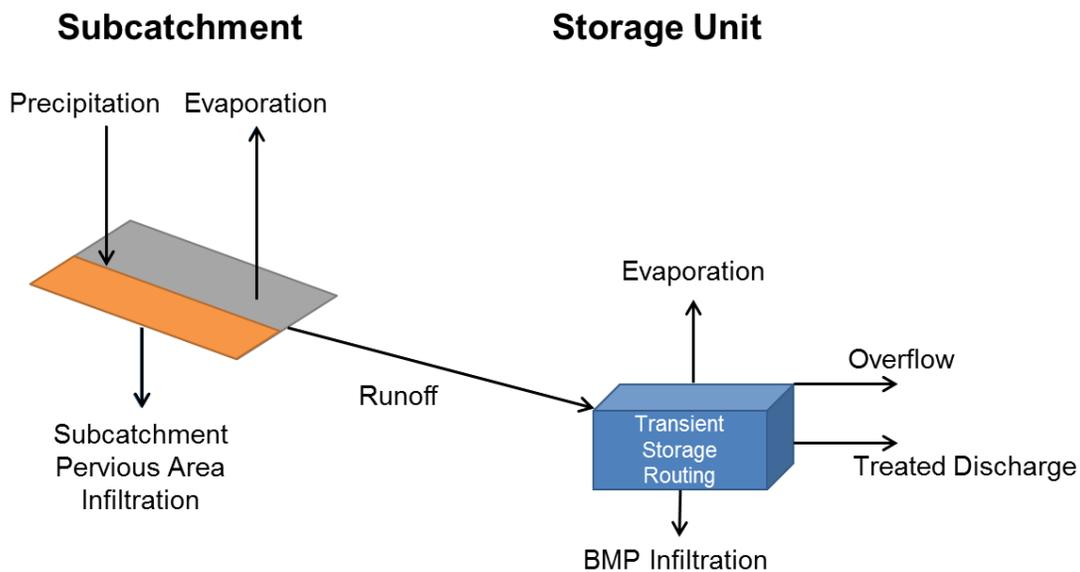
$$\text{Capture Efficiency (fraction of runoff)} = 1 - (\text{Overflow}/\text{Runoff})$$
