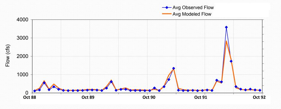
**Modeled Flow vs. Observed Flow**
