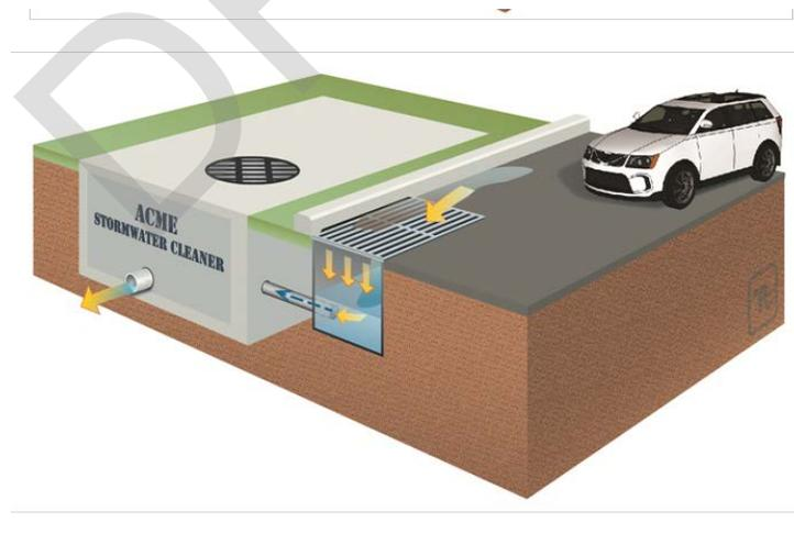
**Figure 3-14: Underground detention schematic**
