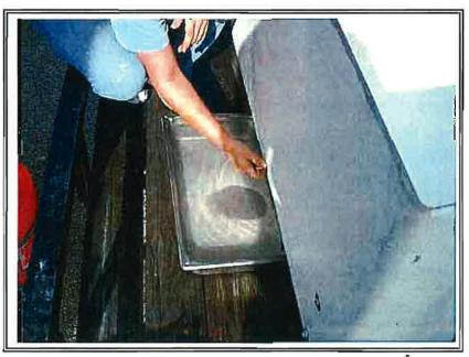
Photo No. 12: Sand in the Curb Inlet testing bed reservoir being washed into a container prior sieve analysis
