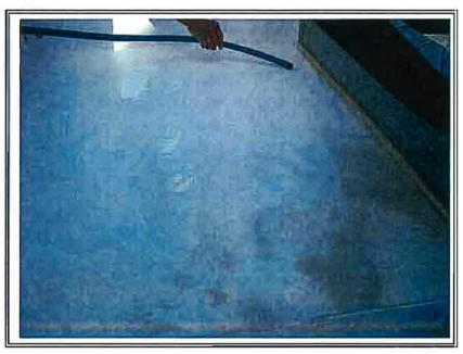
**Photo No. 14**: Sand left in lower tier of Skimmer Box test bed being washed into a container for sieve analysis
