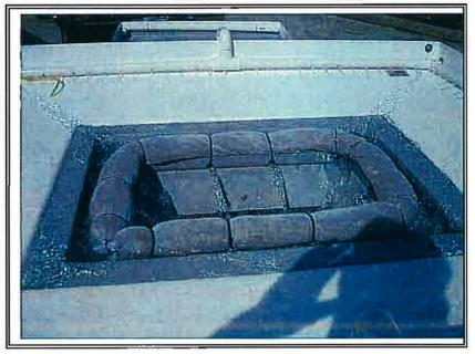
Photo No. 2: Grate Inlet Skimmer Box test bed, upper tier
