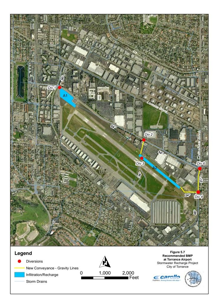
**Option 2**: This is the preferred option. In this option, stormwater diverted from storm drains at Crenshaw Blvd and Amsler Street, and Crenshaw and 250<sup>th</sup> Street will flow by gravity into the infiltration system at Site A3. Stormwater from Crenshaw Blvd. and Amsler Street will be conveyed through a 21-inch pipe to Crenshaw and 250<sup>th</sup> Street. From here, the stormwater will be conveyed through a 24-inch pipe to the infiltration system at Site A3.
