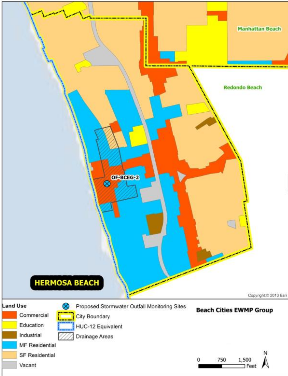
Figure 10 Stormwater Outfall Monitoring Site OF-BCEG-2 Drainage Area
