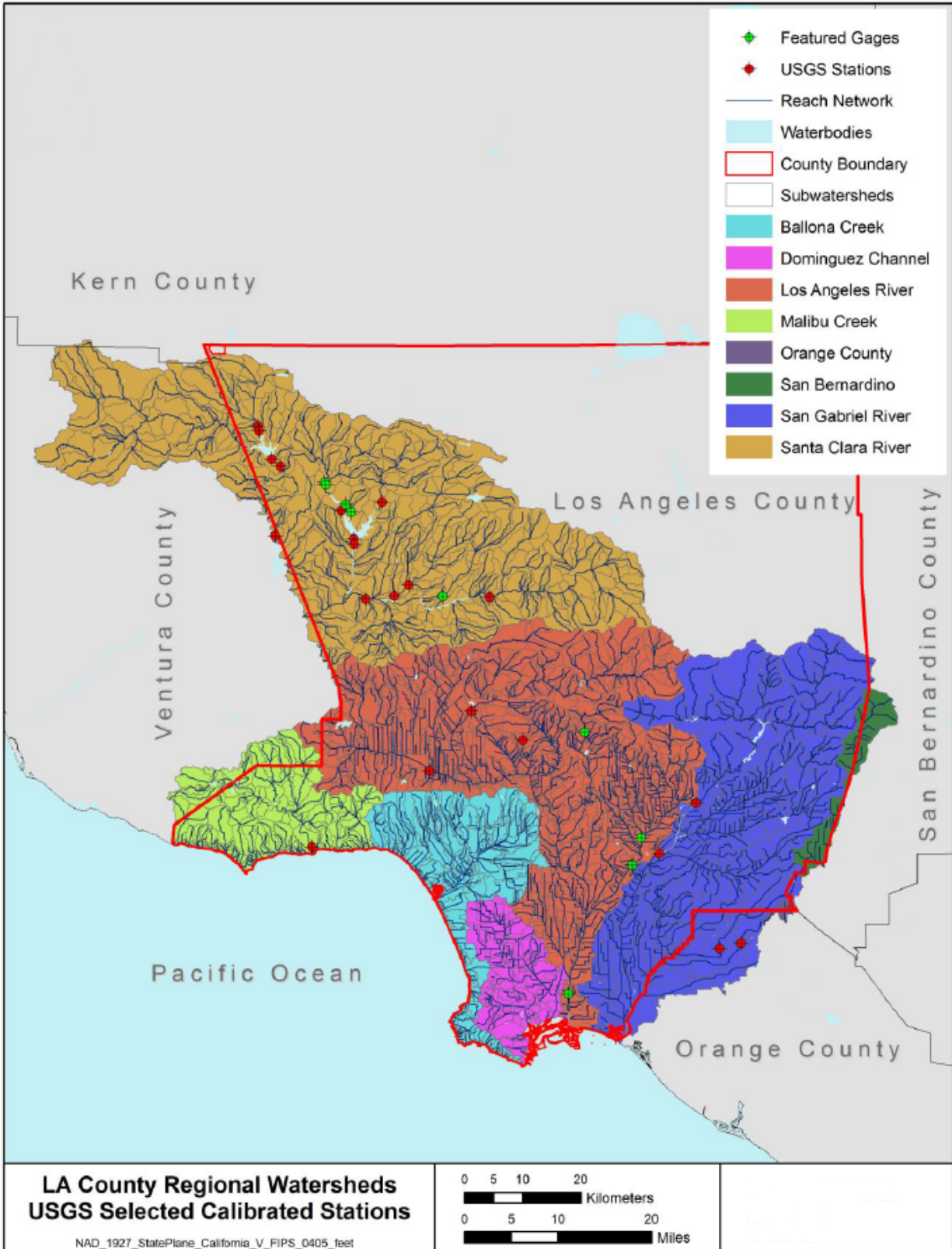
Figure N.3: WMMS/LSPC Runoff Stations used for Calibration (LACDPW, 2010a)
