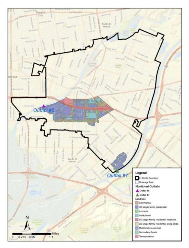
Figure 1-4: Dry and Wet Weather Outfall Drainage Area Land Use
