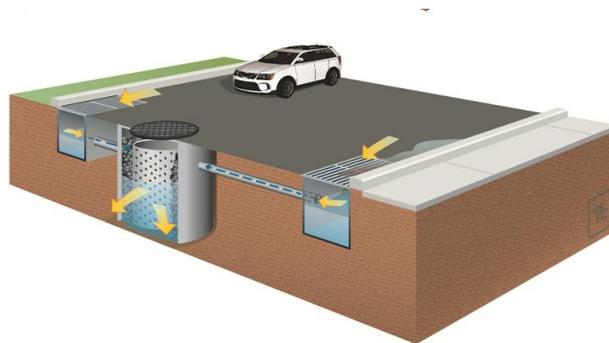
**Figure 3-5: Drywell schematic**
