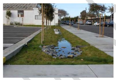
Figure 8: Vegetated swale (Signal hill, CA).
