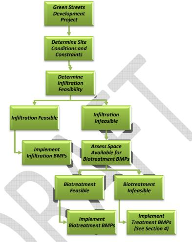
Figure 1: Flow Chart to Determine BMP Selection.
