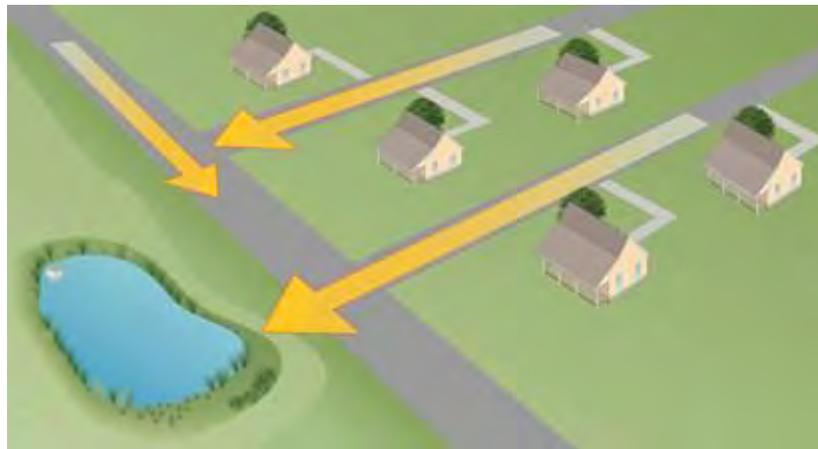
**Figure 3-1 Conceptual Schematic of Regional BMP Implementation Approach**
