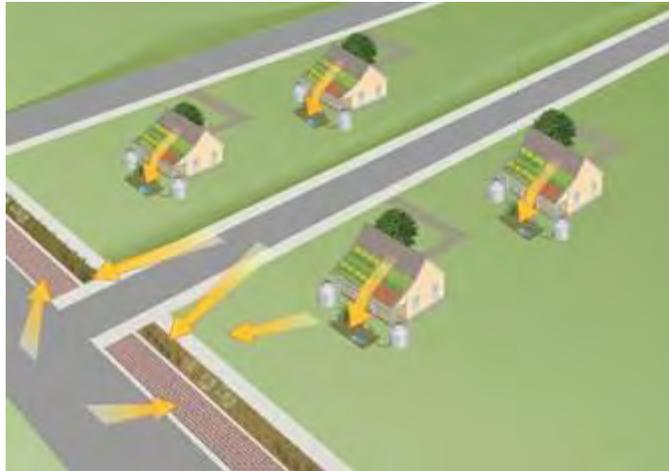
**Figure 3-2 Conceptual Schematic of Distributed BMP Implementation Approach**
