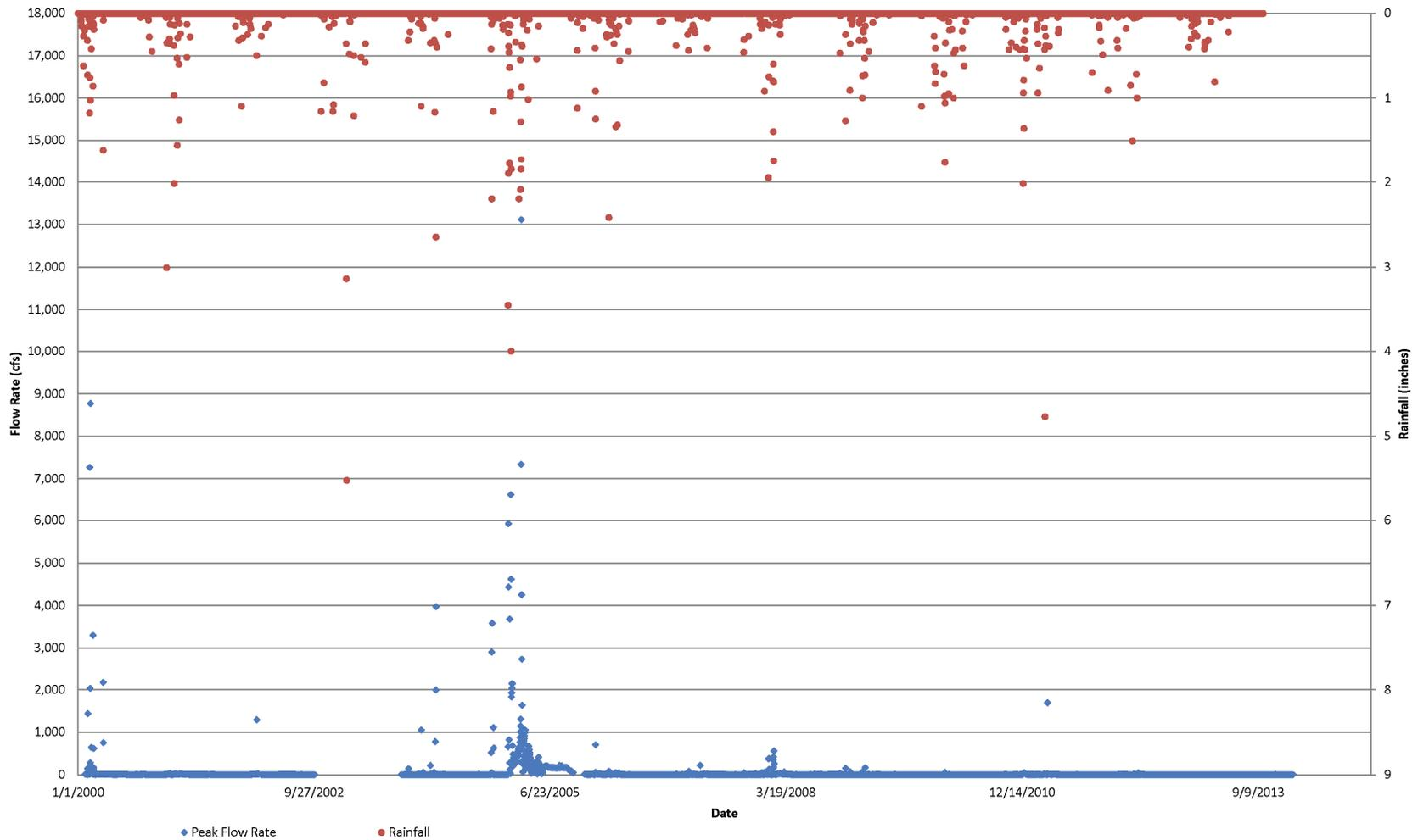
**Figure F-2. Peak Flow Rate and Rainfall Data for Santa Clara River Reach 5 at the Old Road Bridge<sup>2</sup>**
