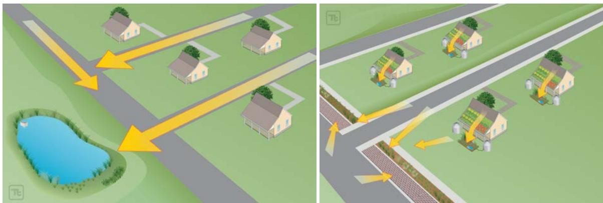
**Figure 5-1. Conceptual schematic of regional (left) and distributed (right) BMP implementation approaches.**
