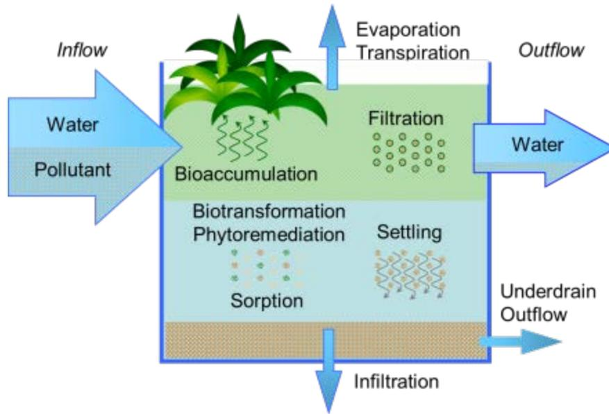
Figure 5-9. Examples of physical processes occurring within structural BMPs
