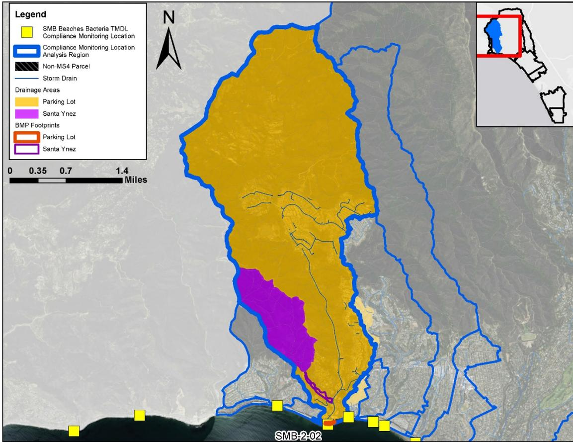
**Figure 8. Modeled Regional/Centralized BMPs within Subwatershed 2-02**
