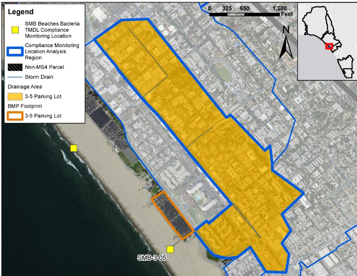
**Figure 15. Modeled Regional/Centralized BMPs within Subwatershed 3-05**
