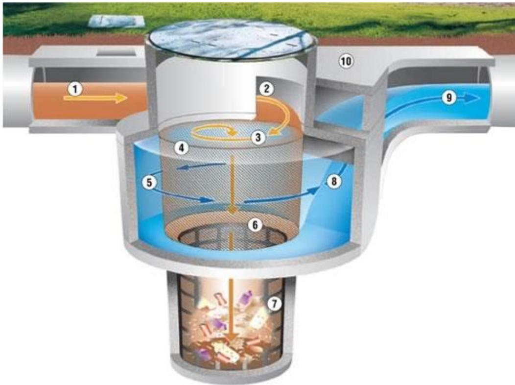
**Figure 6. Example Continuous Deflection Separator (CDS) (image:www.conteches.com)**
