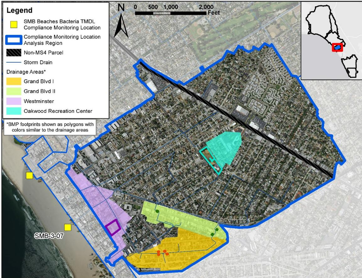
**Figure 17. Modeled Regional/Centralized BMPs within Subwatershed 3-07**
