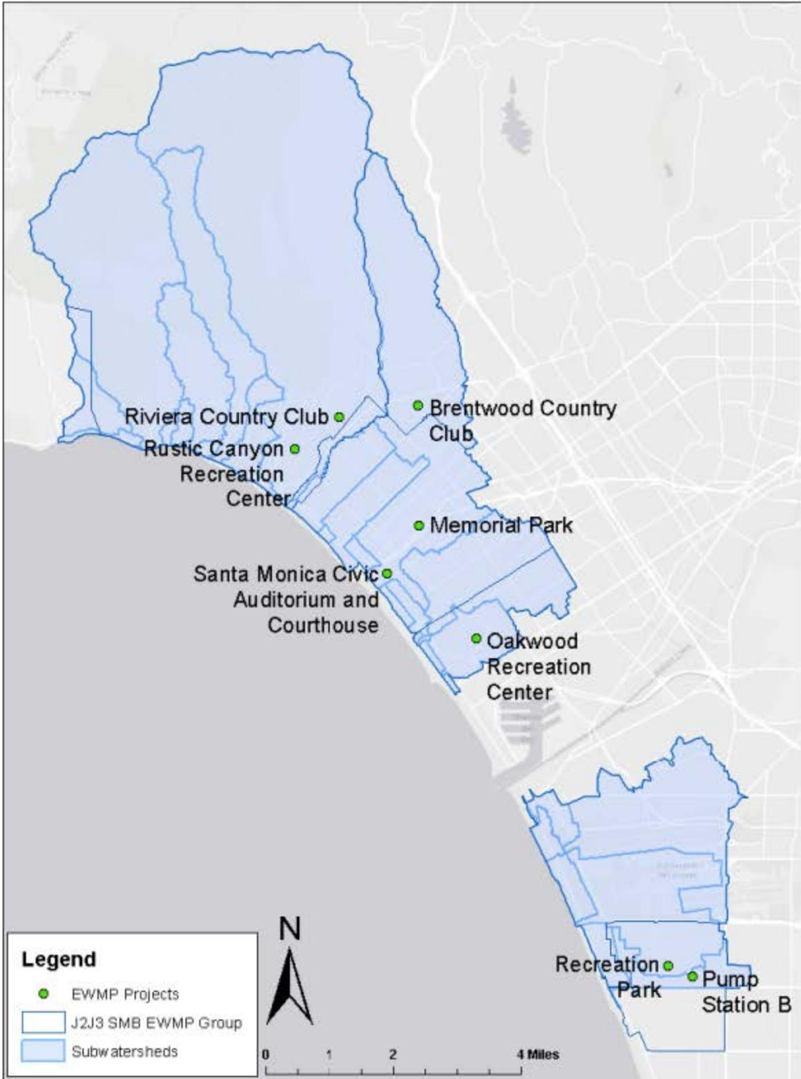
Per Los Angeles' MS4 Permit requirements, all projects were sized to retain and infiltrate the 85<sup>th</sup>-percentile, 24-hour storm event for the drainage area tributary to the project (Regional Board, 2012). Where feasible, BMPs were configured within the site's open areas to avoid removal of trees and existing facilities. Based on discussions with the SMB EWMP Group, the following BMP types were selected:
