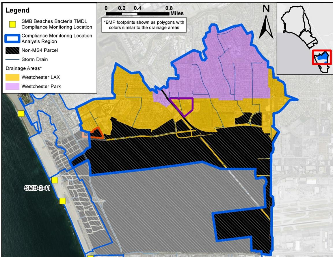
**Figure 19. Modeled Regional/Centralized BMPs within Subwatershed 2-11**
