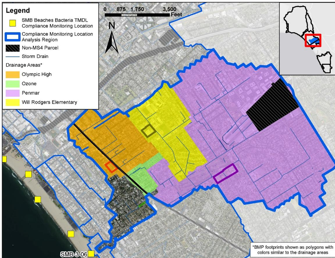
**Figure 16. Modeled Regional/Centralized BMPs within Subwatershed 3-06**
