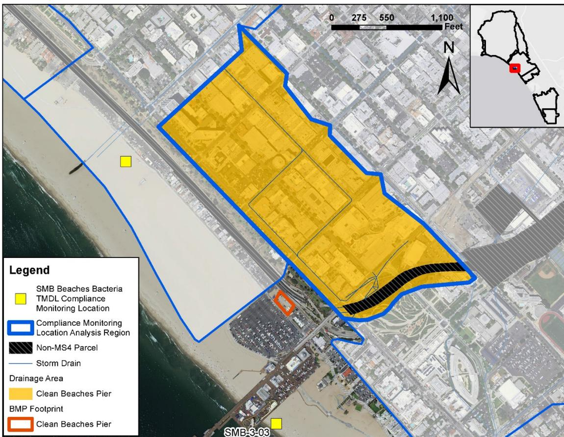
**Figure 13. Modeled Regional/Centralized BMPs within Subwatershed 3-03**
