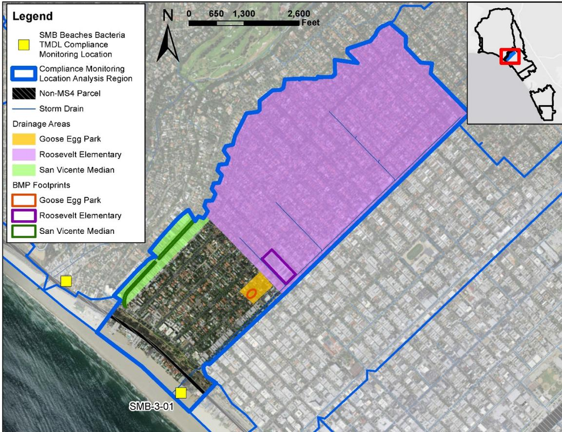
**Figure 11. Modeled Regional/Centralized BMPs within Subwatershed 3-01**
