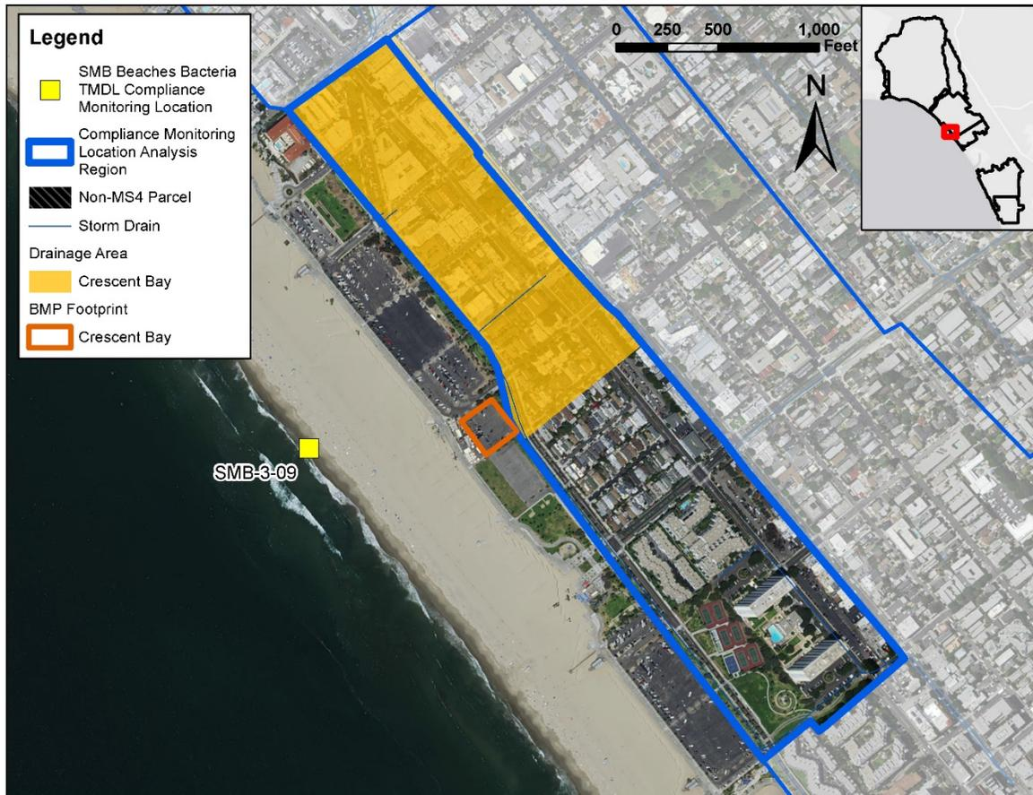
**Figure 18. Modeled Regional/Centralized BMPs within Subwatershed 3-09**
