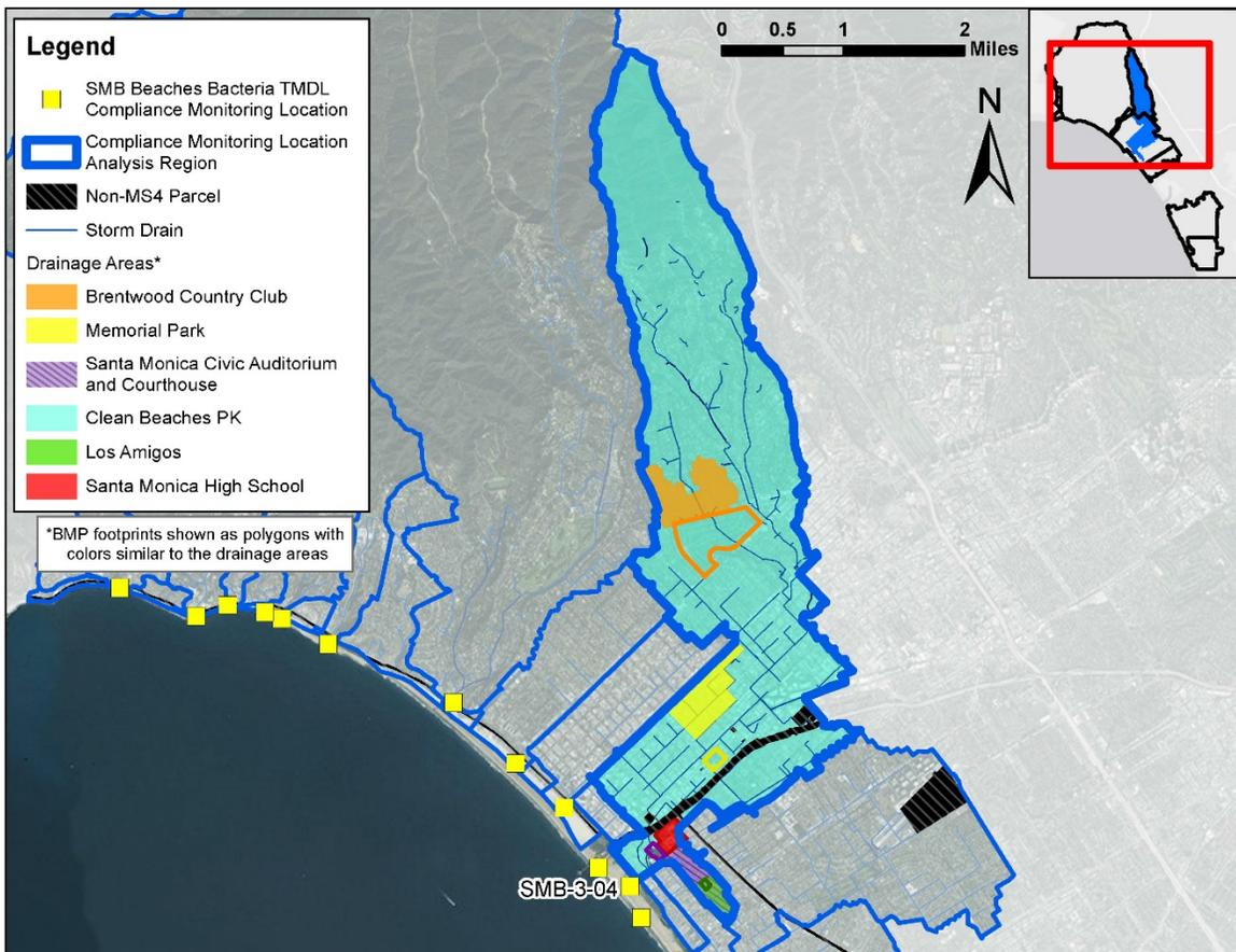
**Figure 14. Modeled Regional/Centralized BMPs within Subwatershed 3-04**
