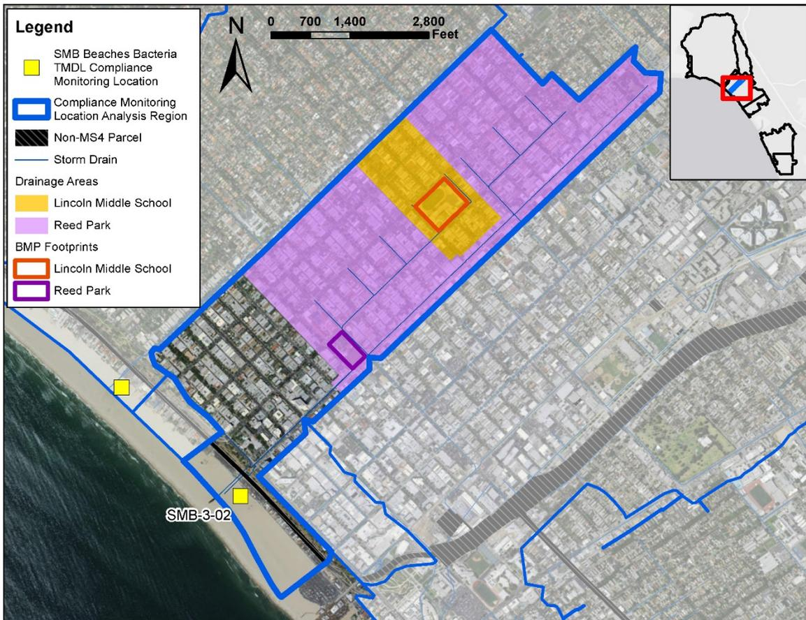
**Figure 12. Modeled Regional/Centralized BMPs within Subwatershed 3-02**
