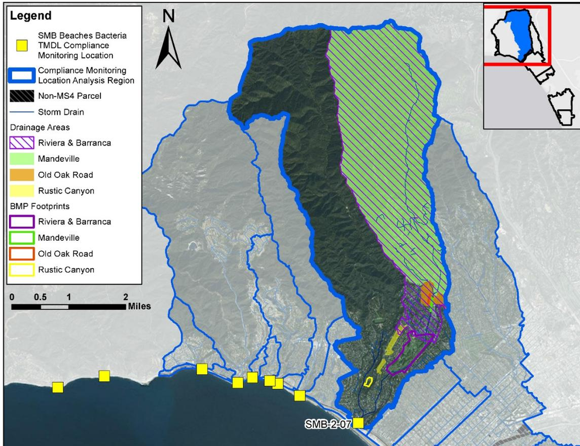
**Figure 10. Modeled Regional/Centralized BMPs within Subwatershed 2-07**
