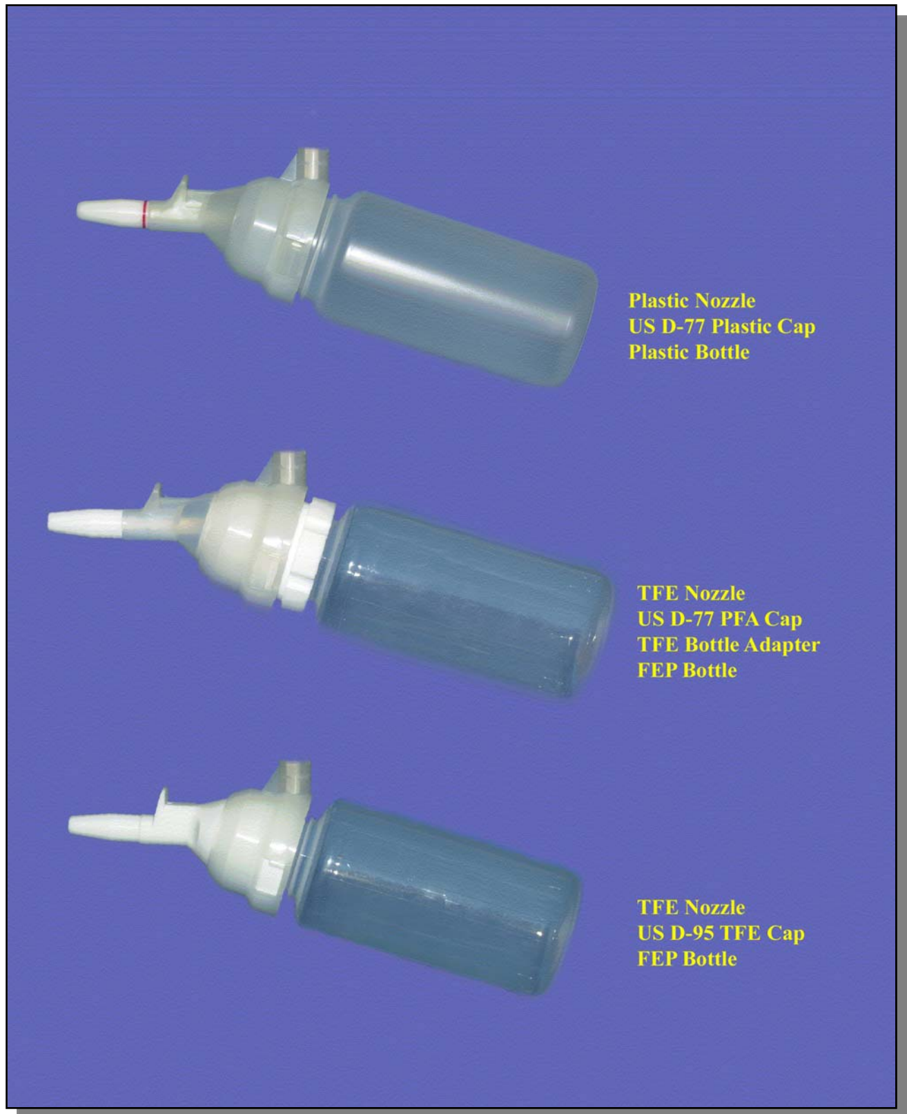
Figure 2. US DH-81 sampler cap/bottle combinations
