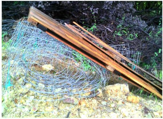
Photo 49-50: Severly weathered sediment control waddles.
