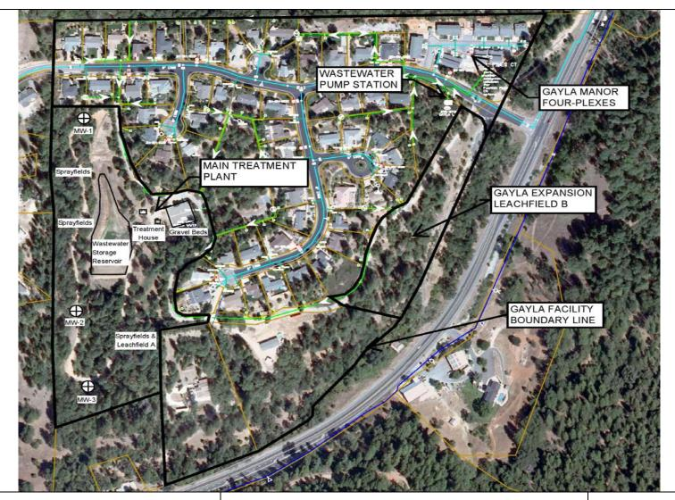
Drawing Reference: RWD supplemental, July 2010 Unknown scale WASTEWATER TREATMENT FACILITY SITE PLAN
