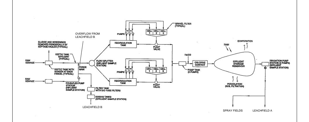
Drawing Reference: RWD Supplemental, July 2010 WASTEWATER TREATMENT FACILITY SCHEMATIC DIAGRAM
