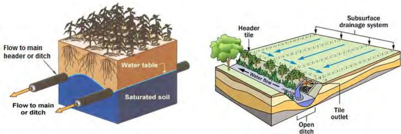
The tile drains are horizontal “pipes”, collecting the irrigation water and shallow groundwater to gravity-fed header tile drains that empty into open ditches or sumps that are pumped into a ditch. Tile drains are placed deep enough below the soil surface (about 7 to 8 feet in the GDA) to keep groundwater out of the crop root zone.
