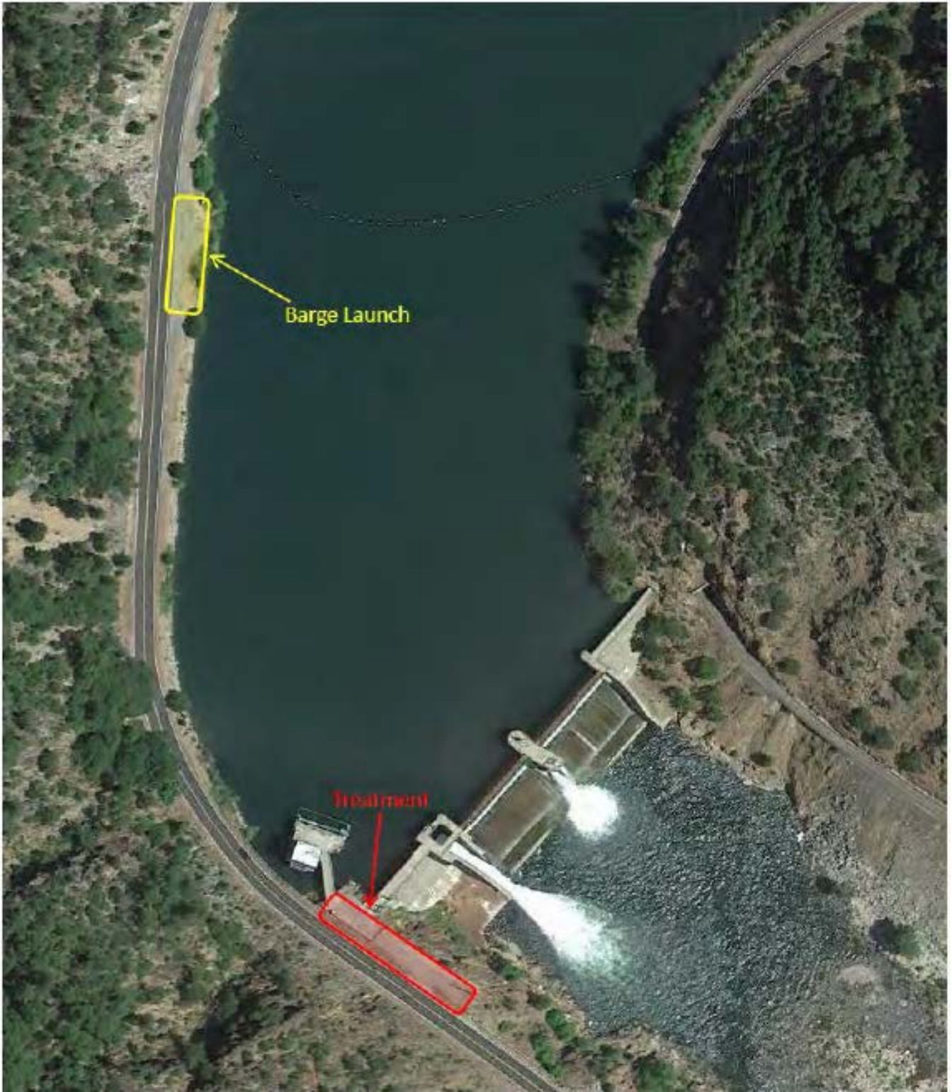
Figure 1: Rock Creek Dam Site Plan
