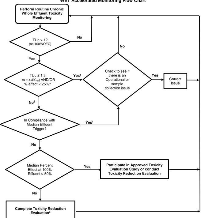
Figure F-2 WET Accelerated Monitoring Flow Chart
