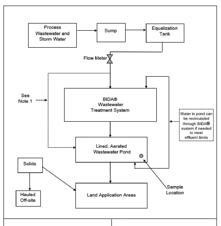
Note 1: Wastewater can be directed to Treatment Pond during period of high flows, such as during storm events, to protect biomass in BIDA® system.
