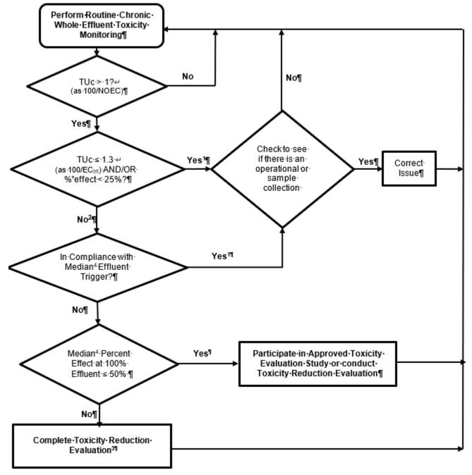
Figure F-1: WET Accelerated Monitoring Flow Chart
