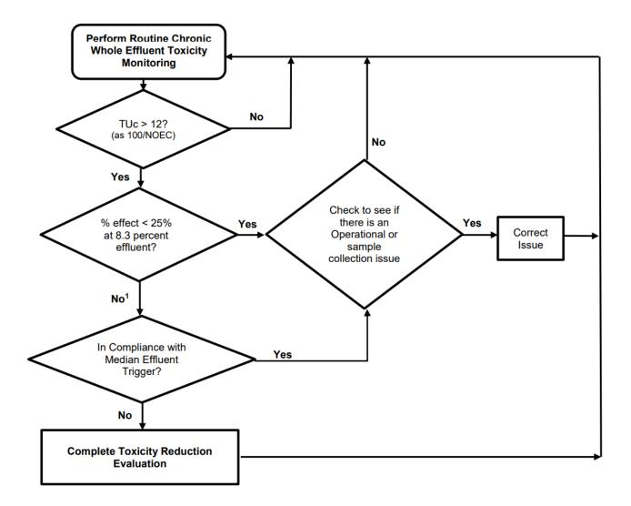
Figure F-1. WET Accelerated Monitoring Flow Chart
