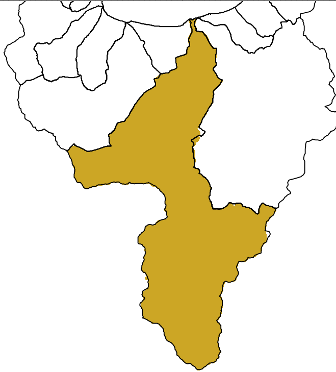
Figure 5-11. The Upper Truckee River generated watershed boundary (black line) and digitized boundary (shaded area).
