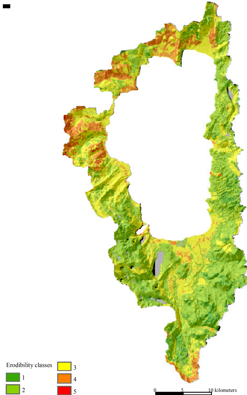
Figure 6-6. Map of upland-erosion potential for the Lake Tahoe Basin obtained by summing the classed values of each of the five selected parameters and reclassifying at a scale of 1 to 5. Areas colored in red and orange represent zones of high upland-erosion potential.
