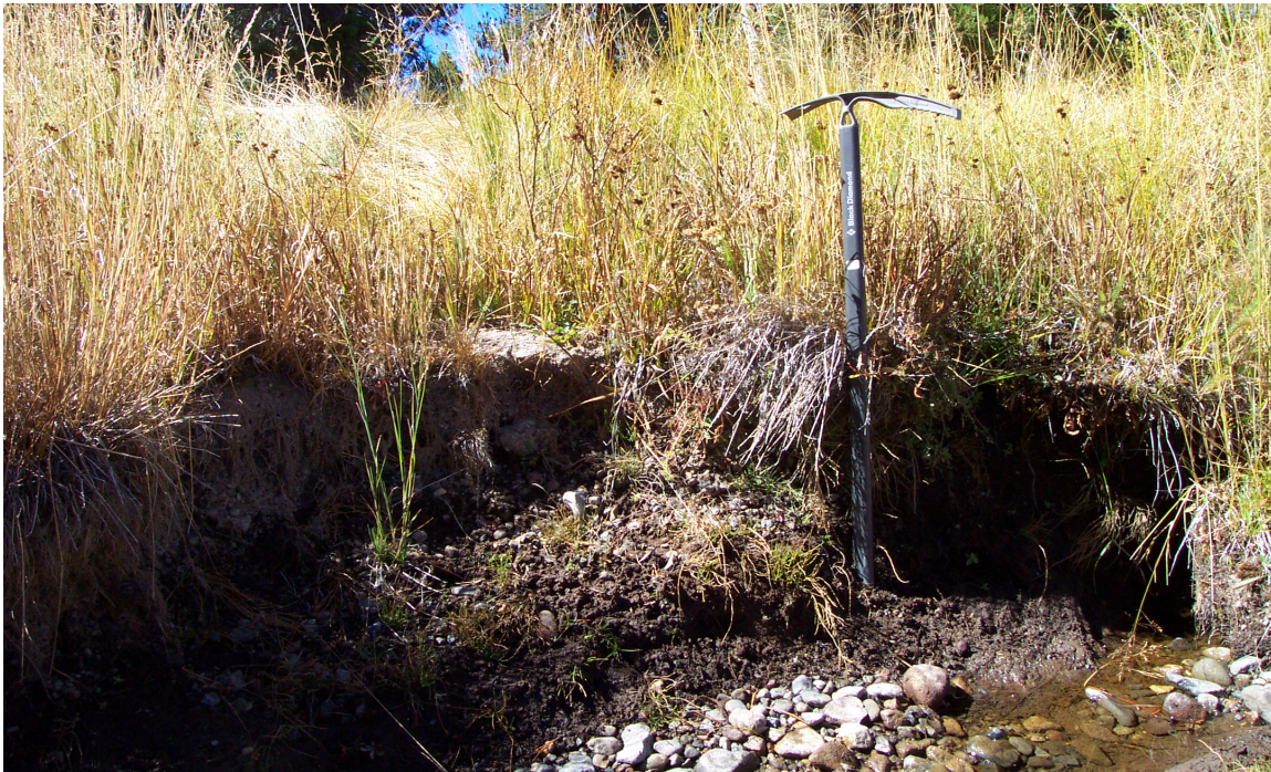
Figure 4-27. Failing bank of fine beaver-pond deposits is rated “low” in fine sediment availability due to low bank height and dense roots fully penetrating bank. The ice axe is 0.75 m tall. Till plain/beaver meadow reach of Ward Creek.
