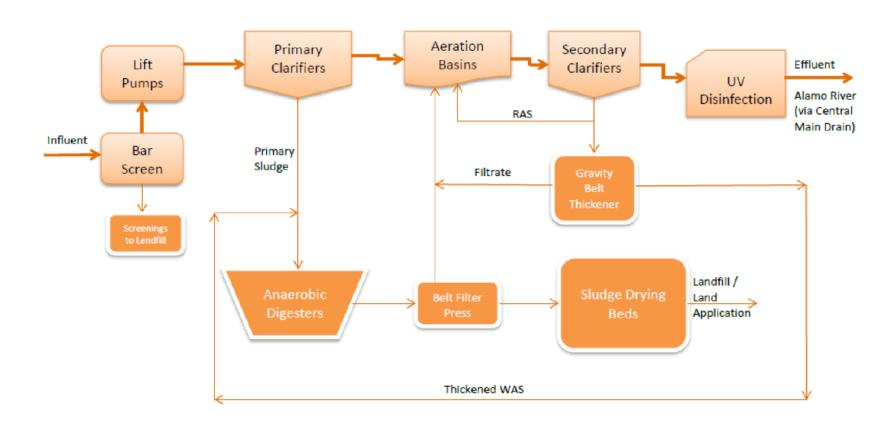
RAS: Return Activated Sludge WAS: Waste Activated Sludge
