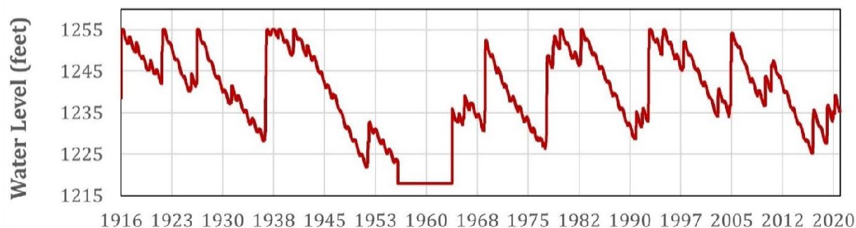
Figure 5-20. Simulated Lake Elsinore Water Level in Reference Scenario (period between June 1956 and May 1964 involved complete lakebed desiccation)
