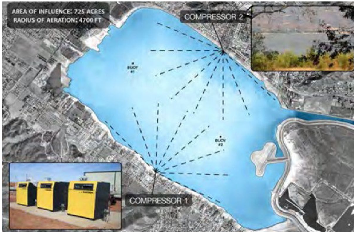
Figure 7-3. Diagram of the Lake Elsinore Aeration and Mixing System (aka LEAMS)
