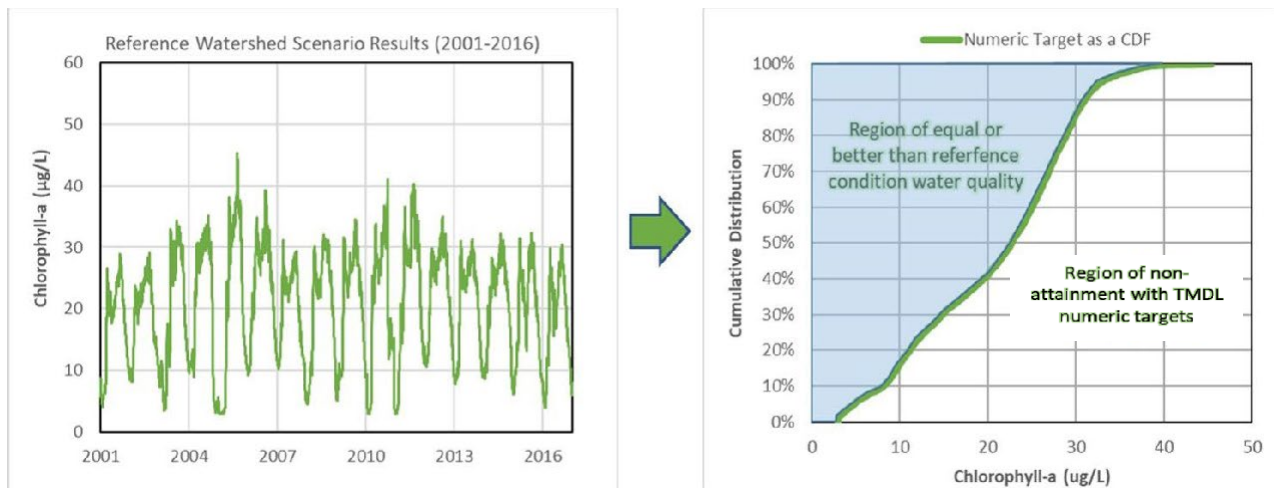
Figure ES-7. Conversion of Dynamic Model Output to a CDF Curve – Example Presented is for Chlorophyll-a in Canyon Lake Main Lake
