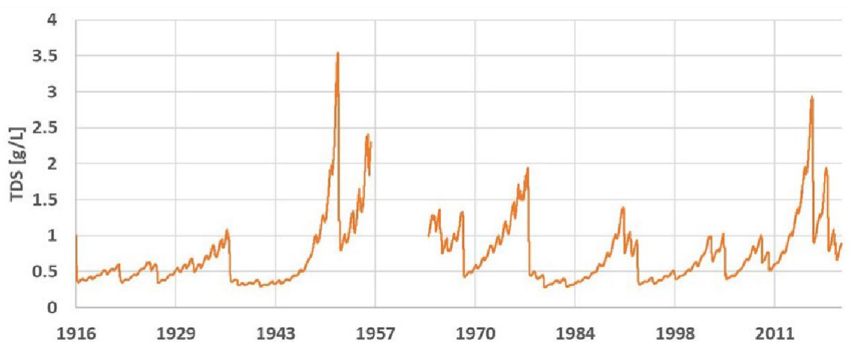
Figure 5-22. Simulated Lake Elsinore Total Dissolved Solids at 2-m Depth in Reference Scenario
