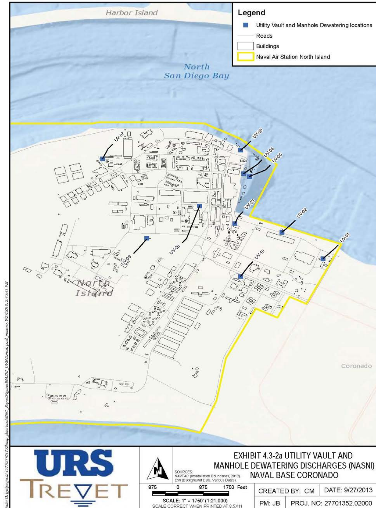
Figure B-6. NBC Utility Vault and Manhole Dewatering Discharge Locations at NASNI
