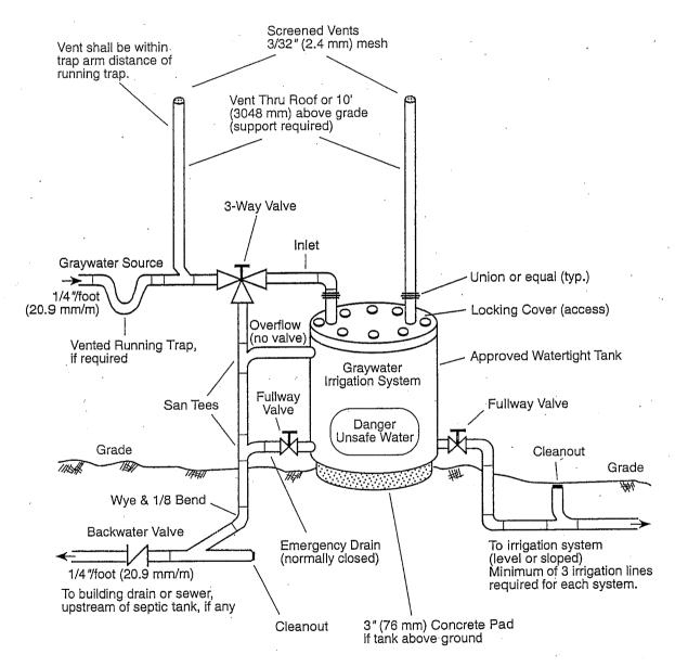
. **Figure G-1** Graywater System Tank – Gravity (conceptual
