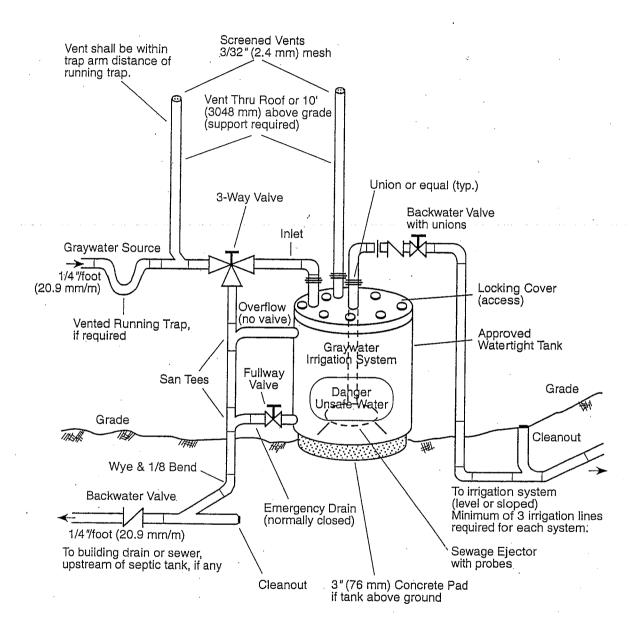
Figure G-2 Graywater System Tank – Pumped (conceptual)
