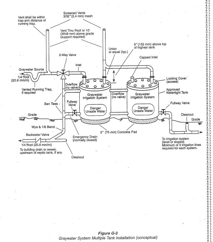
Figure G-3 Graywater System Multiple Tank Installation (conceptual)
