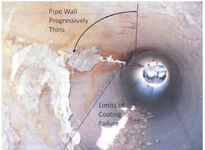
Figure 11. Interior of ruptured forcemain
