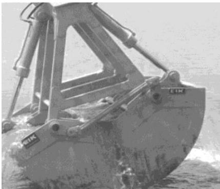
Clamshell bucket to dredge deeper sediments over 25 ft. Bucket dredging is the least desirable for its tendencies to suspend polluted sediments and its excavation inefficiencies.
