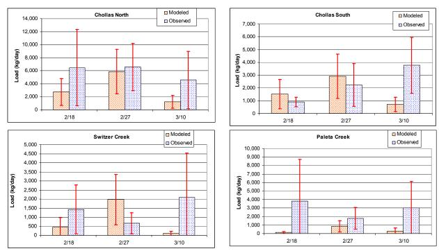
Figure D-17. Modeled vs. Observed Lead Total Storm Loading Comparison
