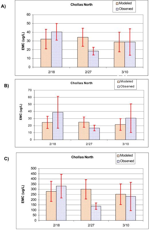
Figure 11. Modeled and measured event mean concentrations (EMCs)  $\pm$  95% confidence intervals for copper (A), lead (B), and zinc (C).
