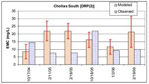
Figure D-20. Validation Modeled vs. Observed Lead Event Mean Concentration Comparison
