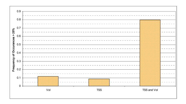
Figure 12. Proportion of storm model simulations (n = 7) that were greater than 25% different from measured values for volume (Vol) only, total suspended solids (TSS) only, and both Vol and TSS.
