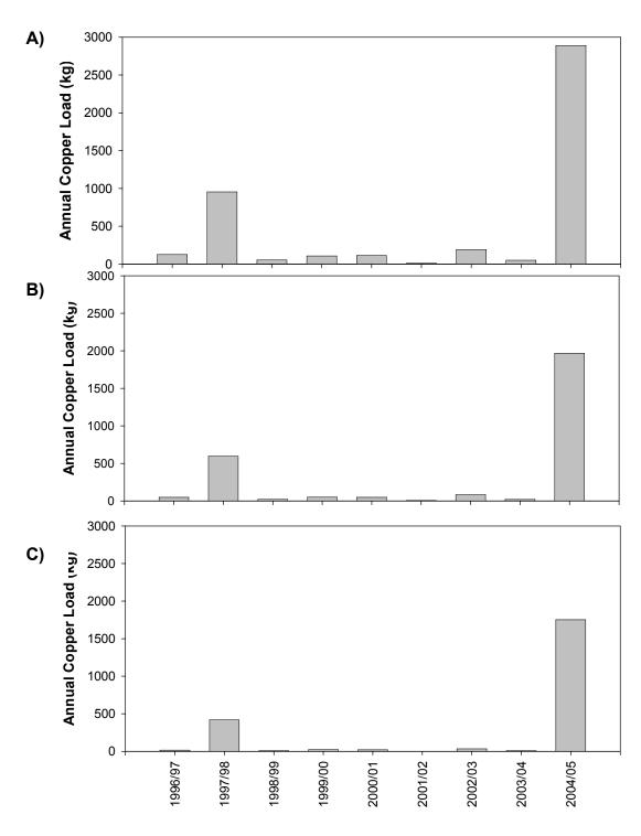
Figure 14. Annual copper loading by water year between 1996 and 2005 for Chollas Creek (A), Switzer Creek (B), and Paleta Creek (C).
