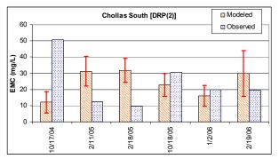
Figure D-19. Validation Modeled vs. Observed Copper Event Mean Concentration Comparison
