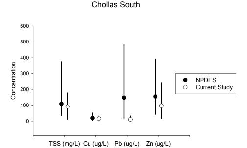
Figure 5. Comparison of min, max, and average concentrations in stormwater from Chollas Creek South from historical data and this study. Historical data courtesy the City of San Diego.
