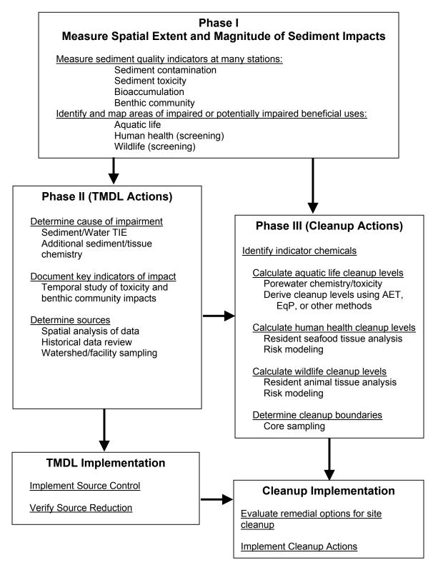
Figure 2. Phased sampling and analysis approach showing the relationship of Phase I sampling plan to potential subsequent TMDL and cleanup activities at the study sites.
