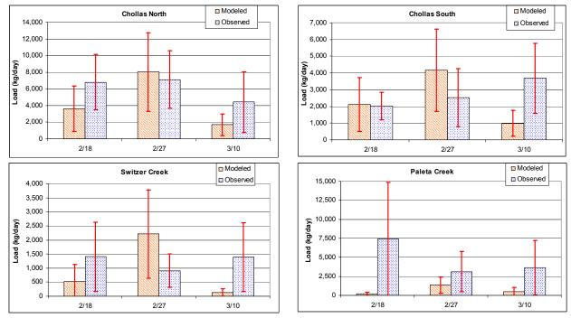
Figure D-16. Modeled vs. Observed Copper Total Storm Loading Comparison
