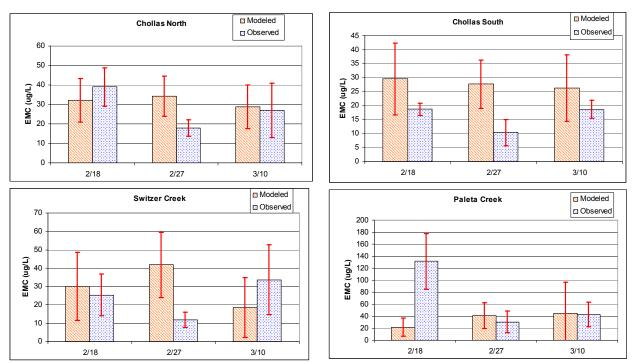
Figure D-13. Modeled vs. Observed Copper Event Mean Concentration Comparison
