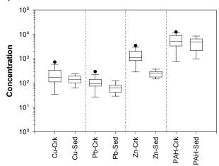
Figure 9. Comparison of TSS normalized stormwater concentrations (-Crk) and sediment (-Sed) concentrations at the Chollas Creek and Paleta Creek mouths. Sediment concentrations from SCCWRP and SPAWAR 2005. Cu, Pb, and Zn (ug/g); total PAH (ng/g).
