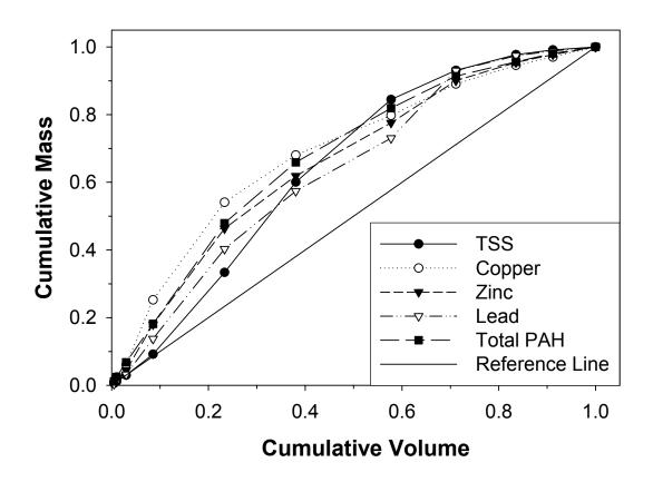
Figure 8. Cumulative mass distribution curves for total suspended solids (TSS), copper, lead, zinc, and total PAH at Paleta Creek, February 27 and 28, 2006. Reference line represents mass acumulation equivelent to flow.
