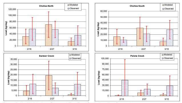
Figure D-18. Modeled vs. Observed Zinc Total Storm Loading Comparison
