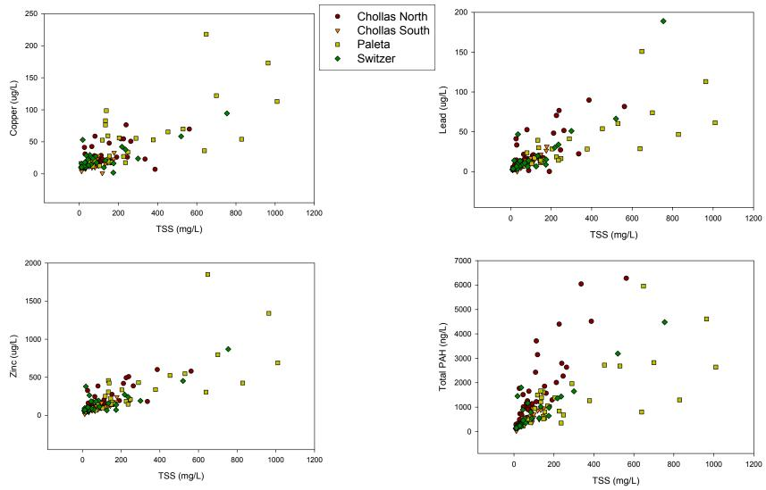
Figure 10. Total suspended solids vs copper, lead, zinc, or total polynuclear aromtic hydrocarbons (PAHs) during wet weather from Chollas North, Chollas South, Paleta, and Switzer Creeks.
