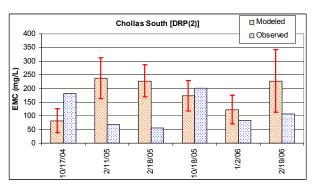
Figure D-21. Validation Modeled vs. Observed Zinc Event Mean Concentration Comparison
