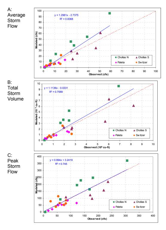
Figure 11. Modeled versus observed results at Switzer, Chollas North, Chollas South, and Paleta Creeks.
