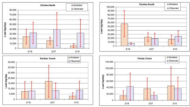
Figure C-5. Modeled vs. Observed TSS Total Storm Loading Comparison
