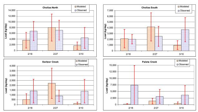
Figure C-6. Modeled vs. Observed Copper Total Storm Loading Comparison
