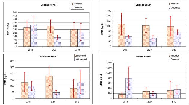
Figure C-4. Modeled vs. Observed Zinc Event Mean Concentration Comparison
