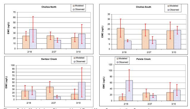
Figure D-14. Modeled vs. Observed Lead Event Mean Concentration Comparison
