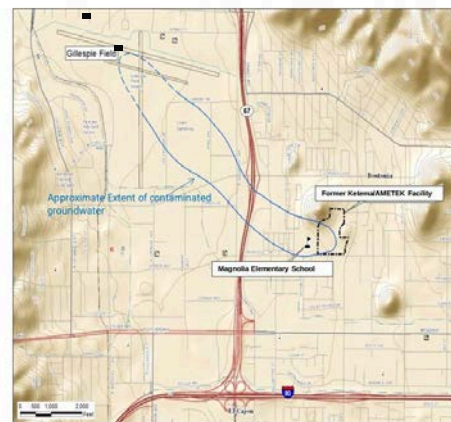
Figure 1: Former Ketema/AMETEK Facility Location and Extent of Contaminated Groundwater
